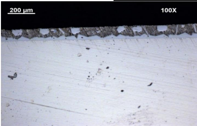
Figure 5. Microstructure of non-diffused sample 10% Al-Si
